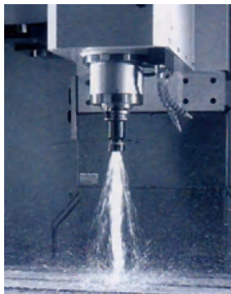
Spindle center water outlet
